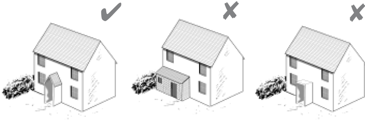
Figure 10: Acceptable and unacceptable front extensions
